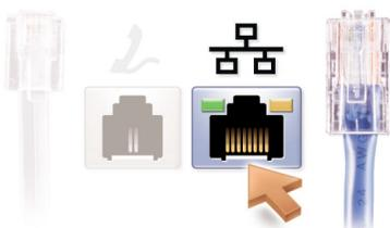
To use the network adapter, connect a separately purchased network cable to the network connector.
