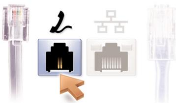
To use the internal modem, connect the telephone cable to the modem connector and connect the other end of the cable to a telephone wall jack.
